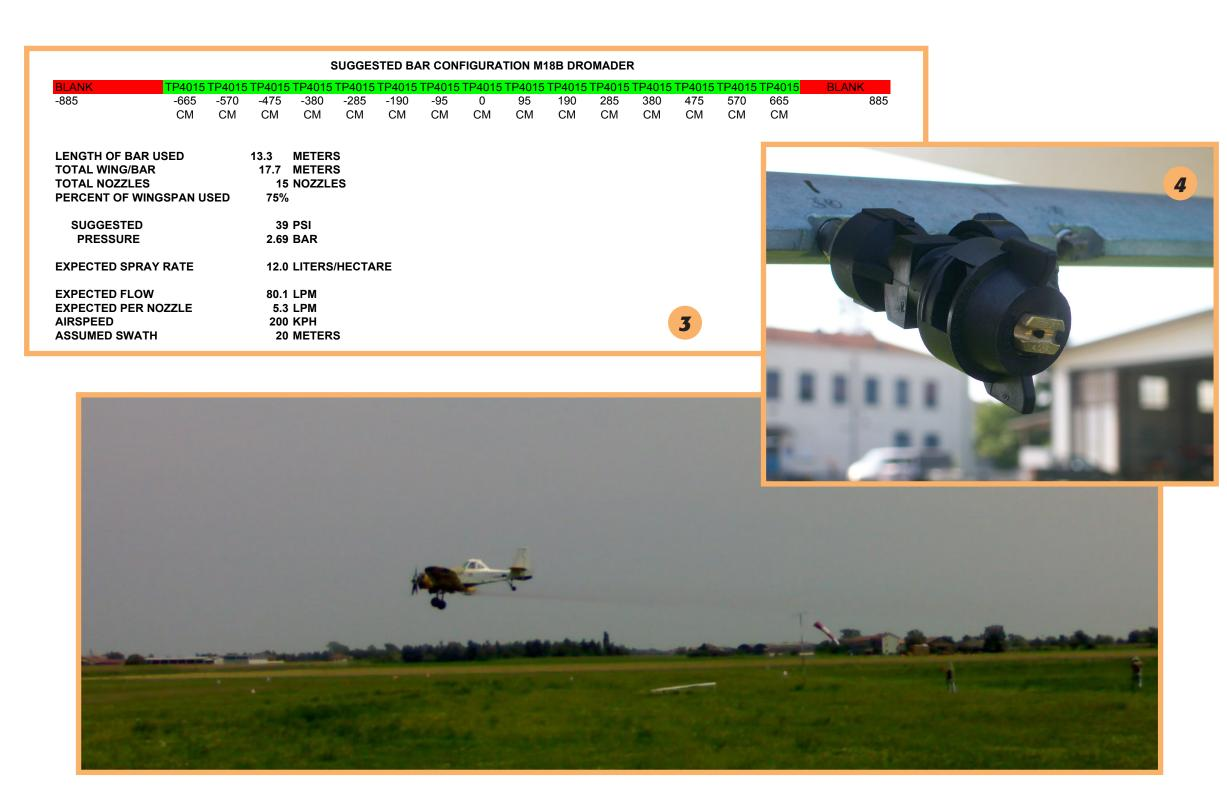
psi (2.69 bar) were mounted with an angle of 0 degrees respect the air-stream, straight-back and parallel with ground (Fig. 4). The nozzles were mounted on each boom at 0, 95, 190, 285, 380, 475, 570 and 665 cm from the centre of the fuselage.
